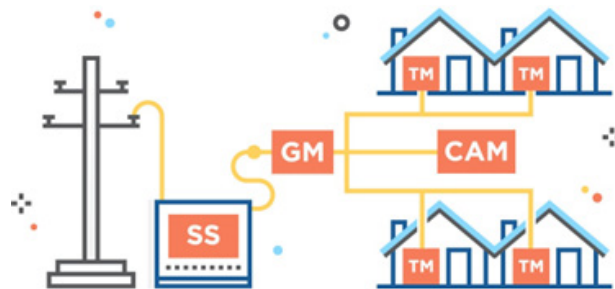
SS: Sub-Station GM: Gate Meter CAM: Common Area Meter TM: Tenancy Meter
